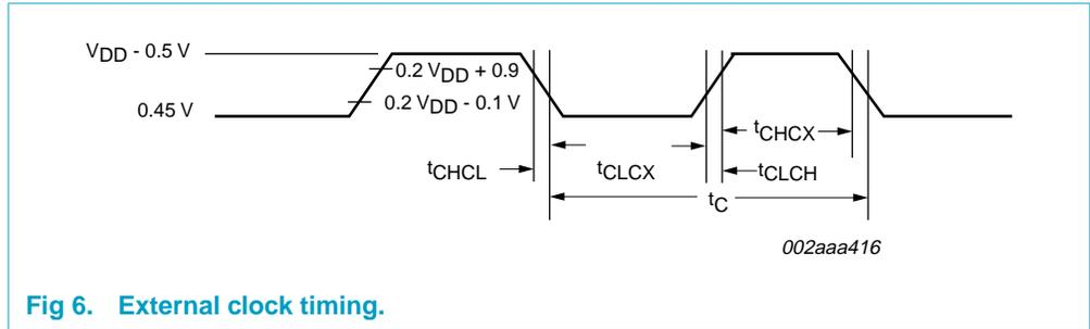
Fig 6. External clock timing.
